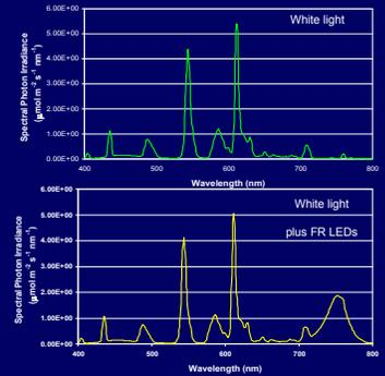
Figure 6. Spectral energy distributions of control and far-red-supplemented growth cabinets
