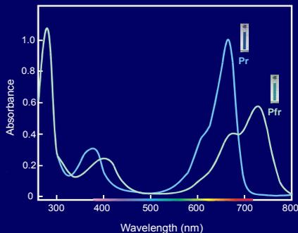
Figure 2. Absorbance spectra of the Pr and Pfr forms of phytochrome
