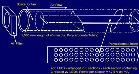
Figure 3. Design of far-red LED arrays
