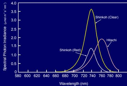
Figure 1. Spectral characteristics of far-red LEDs
