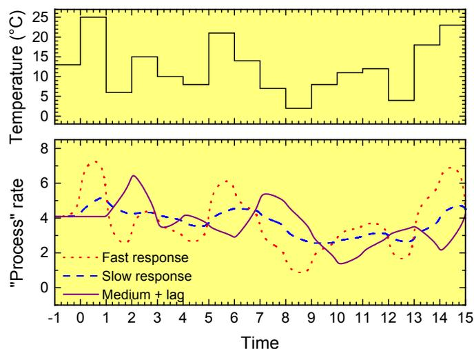
Fig. 14. An hypothetical example of varying temperature in pseudo-random steps and how changes in plant processes that vary in rate might occur in response to the stepped change©.
