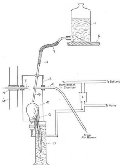
Fig. 7. Details of humidifier. A, tin; B, 8 candle-power carbon filament lamp; C, muslin covering lamp loosely; D, cylinder for water; E, air inlet to tin; F, air exit to chamber; G, tube to lead drip to lamp; H, drip jet; I, connecting tube to reservoir; J, water reservoir; K, bracket screwed to top of chamber; L, relay; M, glass walls of chamber; N, side rail of chamber.
