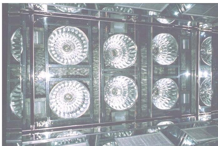
Fig. 6 The water-screened high-light rig at the NZ Controlled Environment Laboratory using High pressure discharge and tungsten halogen lamps©.
