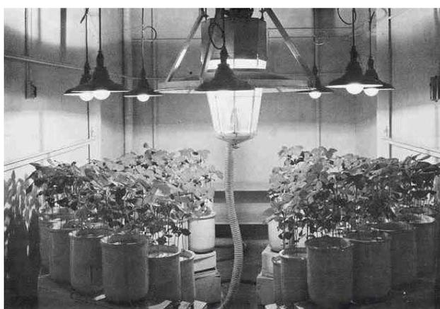
Fig. 3 An example of the carbon arc lamp (from Downs 1980).
